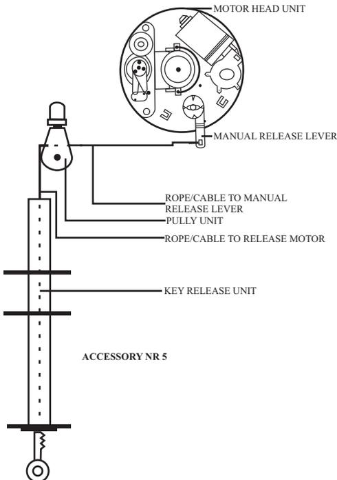
1. Drill 20mm hole through wall next to door, eye level on the side where the motor is situated.
